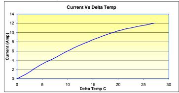
Note: Delta temp= Cut-off temp at No-load - Cut-off temp at rated Current
